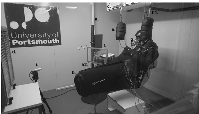
Fig. 1. The flight environment simulator: (a) Custom-welded hollow steel frame; (b) Semirecumbent cocoon harness; (c) Cooling system; (d) Fan unit; (e) Down sleeves, containing weighted brake lines and brake handles; (f) Computer monitor, Perspex shield, enlarged keyboard and stylus; (g) Metamax 3b; (h 1-2) Ambient temperature sensors; (i) Monitoring camera; (Out of shot) Projector and chase cam video, oxygen saturation logger with ear probe, skin and rectal temperature sensors.
