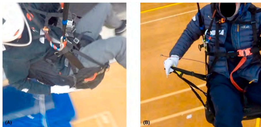
Fig. 6. (A) Participant's first attempt to locate the reserve handle is on his hip, despite that being significantly behind the handle's actual position. (B) Participant grabs his reserve handle, and his harness stirrup at the same time, is unable to the extract the deployment bag and fails to deploy.
