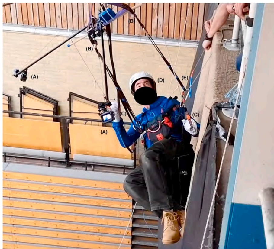
Fig. 2. Zipline set up in the moments before release for a participant with a front-mounted system. (A) Cameras; (B) LED lights; (C) Hands in control lines responding to the light sequence; (D) Gaze directed upwards; (E) Tensioned release.
