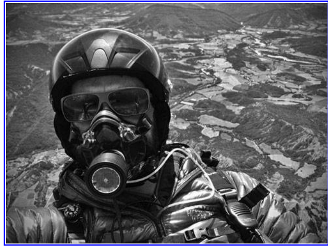
FIG. 2. Phases of flight: Author M.W., testing the ME-TAMAX 3B in flight at 2200 m over Laragne-Monteglin, France.
